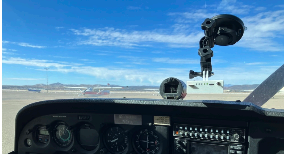
Figure 9: Example installation of OnFlight Hub aligned with aircraft reference frame.
